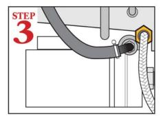
Connect the glasswasher to a 120-140°F hot water source. The minimum temperature will remain in the wash cycle until the booster heater reaches 180°F; then it will advance into the rinse cycle.
