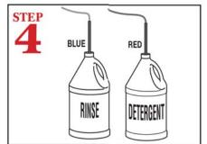
Insert the chemical tubing into the tube stiffeners, and then insert tube stiffeners into the corresponding chemical dispensers.
